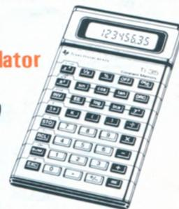
This powerful 54-function calculator performs most-needed slide rule functions as well as pi, factorial & constant. LCD display with scientific notation. Built-in statistical capabilities include data entry, mean & standard deviation for both sample & population data. Versatile 4-key constant memory feature lets you store, recall, sum & exchange memory with display. Includes the "Student Calculator Math Book", detailed Owner's Manual & vinyl carrying case.
